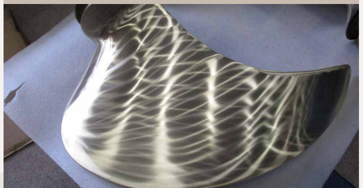
4. Honed, and the repair is completed
